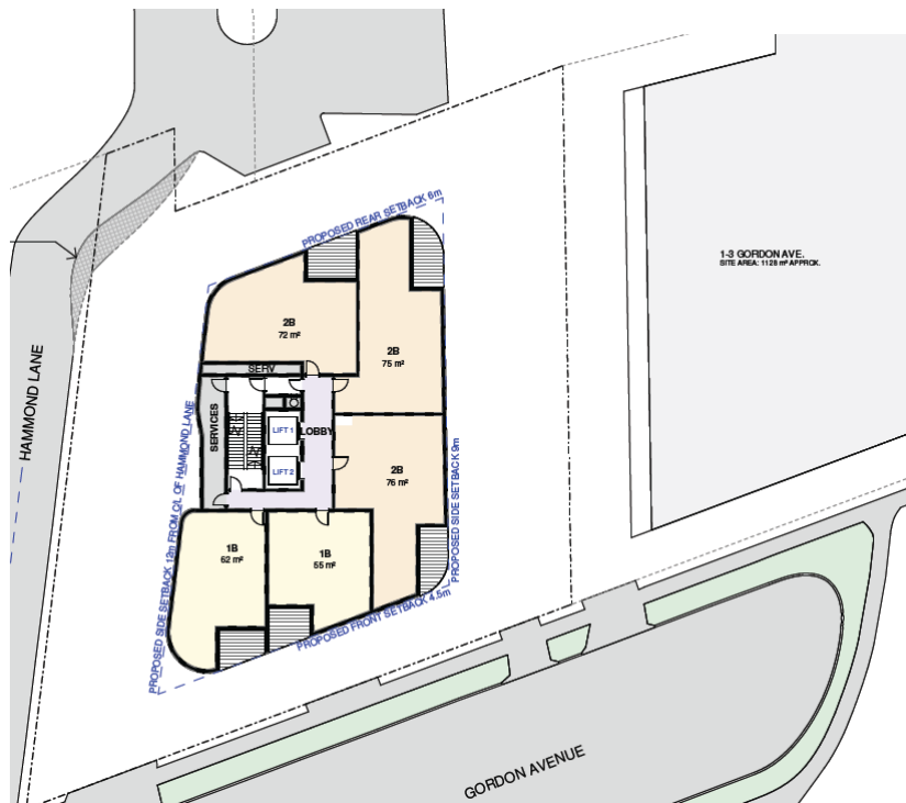
Figure 18 - Typical 400m 2 (GFA) Tower Floor Plate Levels 3-17
